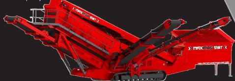
The Maximus 518T has a highly aggressive, heavy duty, 2-bearing, 18ft x 5ft (5.5m x 1.525m) 3 deck screenbox with class leading screening area and output potentials.
